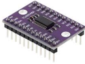
Figure 3.5: The TCA9548A 8-channel I2C multiplexer module, used to resolve sensor address collisions.
