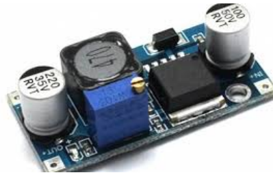
Figure 3.8: The LM2596 step down (buck) converter module, utilized for high efficiency 3.3V voltage regulation.
