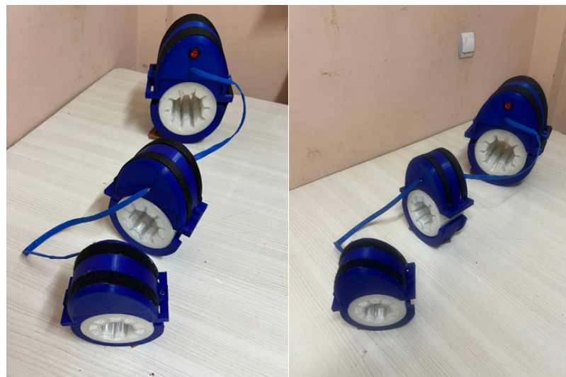
Figure 3.14: Z: The fully assembled physical prototype of the multi-segmental kinematic tracking system, featuring the rigid outer enclosures, the flexible TPU biomechanical interface (white inserts), and the inter-node wiring.
