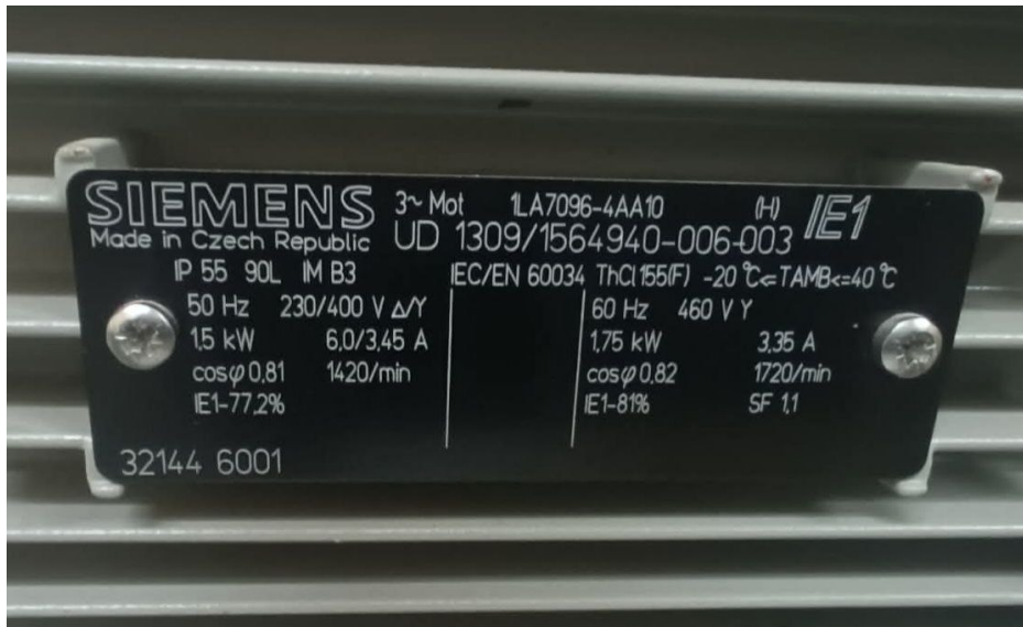
Figure 2.1: Nameplate of the Siemens 1LA7096-4AA10 laboratory induction motor.
