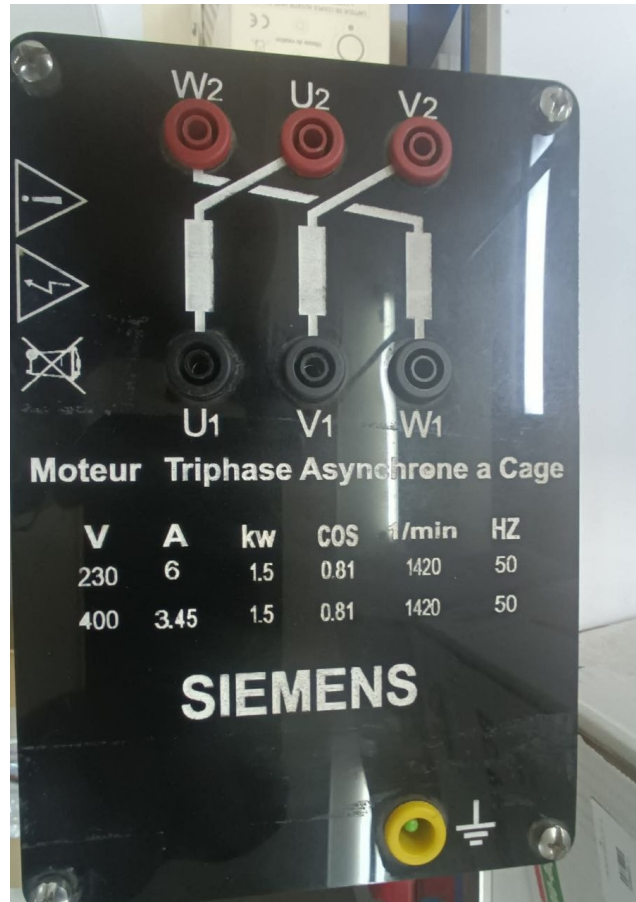
Figure 2.2: Terminal-board plate of the Siemens laboratory motor showing the 230/400 V, 1.5 kW ratings.
