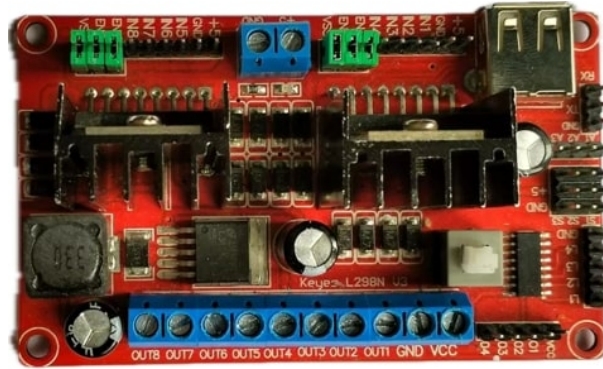
FIG. 2.23 – L298N Motor Driver
