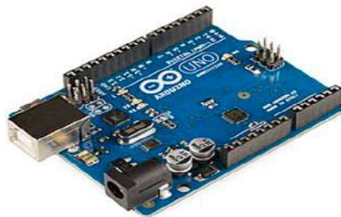
Figure I. 13 - Arduino Uno development board based on the ATmega328P microcontroller
