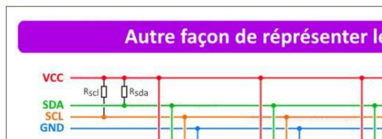
Figure V. 10 - Alternative representation of the I 2 C bus
