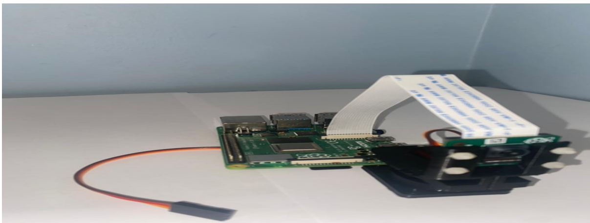
Figure 5.30: Assembly of Raspberry Pi 4, Camera Module v2, Gimbal, and Servo Motor Components
