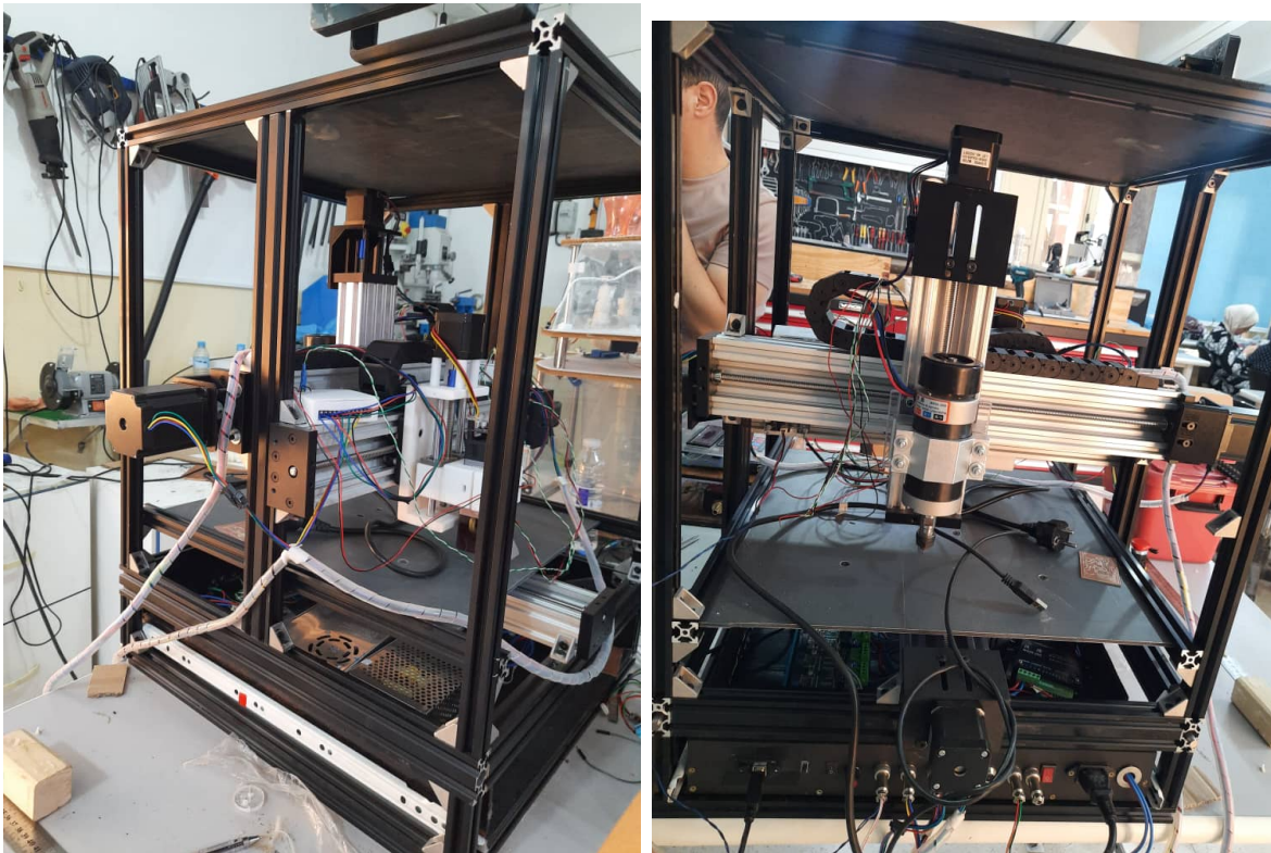
Figure 3.21 The full assembly of the CNC machine.
