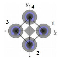
FIGURE 2.2: Direction of propeller's rotations
