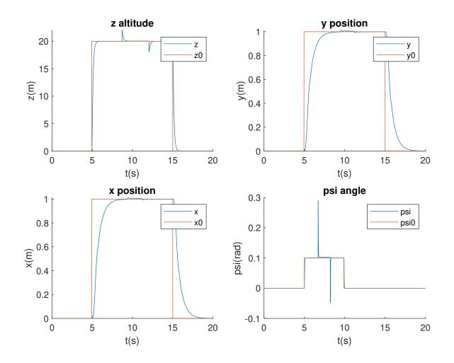
FIGURE 4.4: xyz positions and the yaw angle  $\psi$  with disturbances
