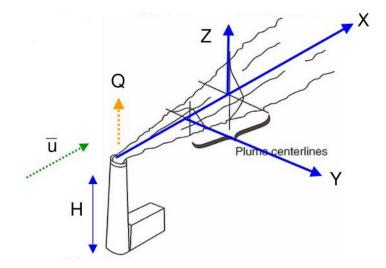
FIGURE 3.4: Gaussian plume model
