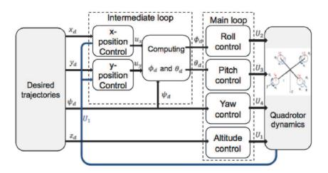
FIGURE 2.8: Structure of a quadrotor strategy control
