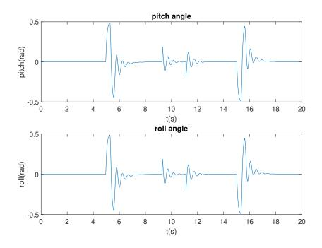
FIGURE 4.5: Pitch and roll angles  $\phi, \theta$  with disturbances
