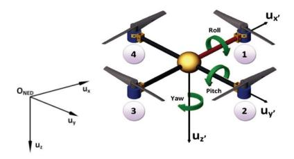
FIGURE 2.7: Quadcopter configuration
