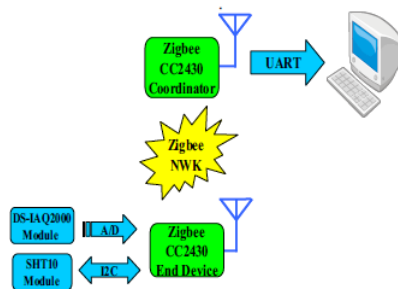
FIGURE 1.6: General architecture of outdoor AQM System Based on ZigBee Wireless Sensor Network
