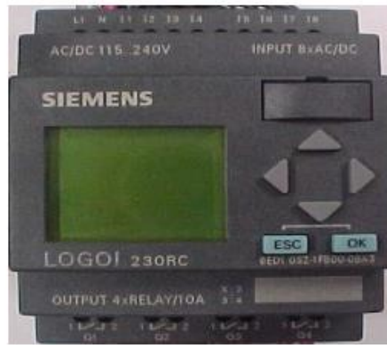
Figure III. 1: PLC de forme compacte(fixe) [25].
