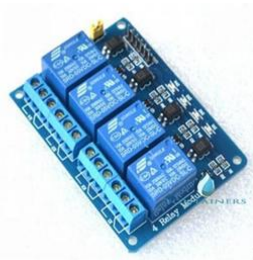
Figure III-10 Le relai SRD-05 VDC-SL-C
