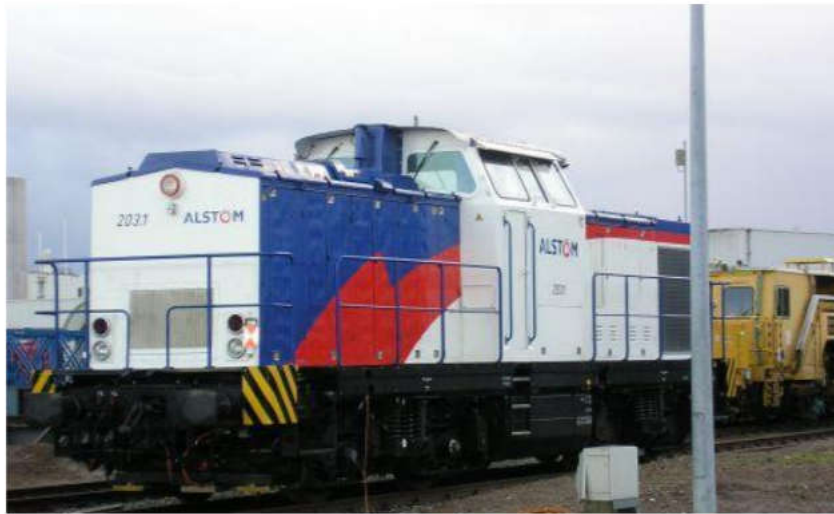
Figure 1.7 : Locomotive hybride BR203 de RailPower (ALSTOM)
