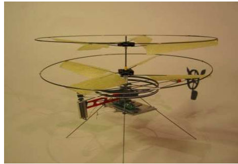
Figure I. 5 : Le PicoFlyer (ProxyFlyer)
