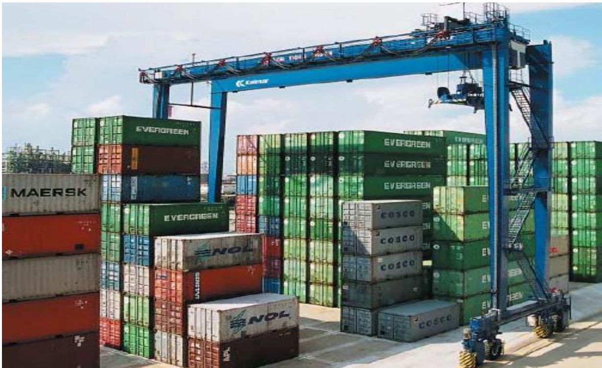
Figure II-15 Grue Kalmar RTG
