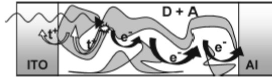
Figure II-6: volumetric heterojunction cell structure
