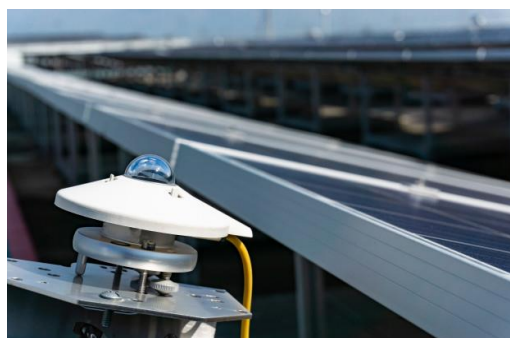
Figure I-8: Pyranometer for Measuring the irradiance of a Solar Farm, in a Solar Cell Factory
