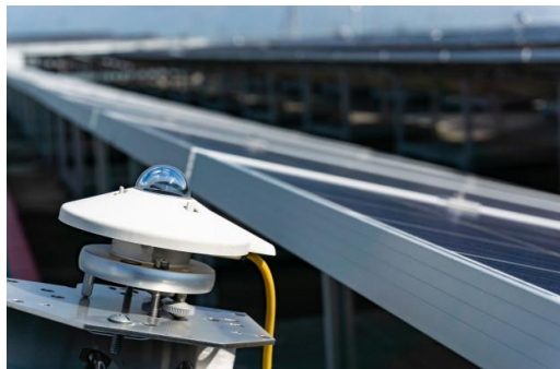
Figure 8: Pyranometer for Measuring the irradiance of a Solar Farm, in a Solar Cell Factory
