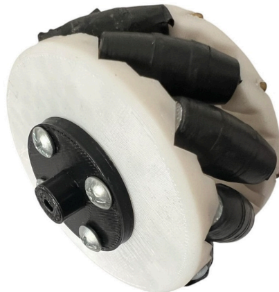
Figure 4.6: Detailed View of 3D Printed Mecanum Wheels
