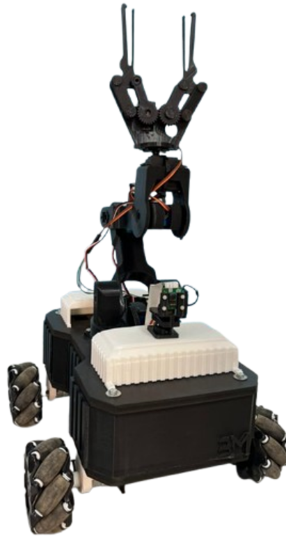
Figure 4.11: Assembled Mobile Robot Manipulator
