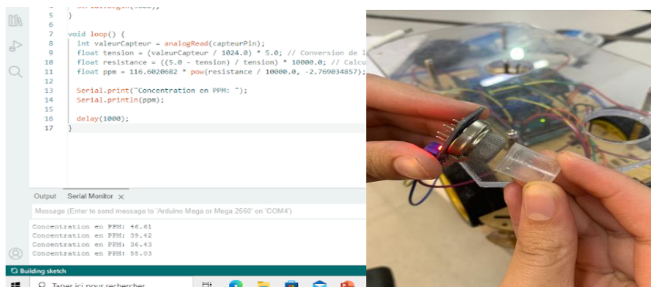
Figure III.16 Images of the tests of the MQ135 sensor
