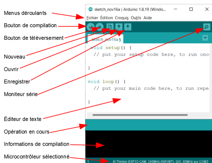
Figure II.12 Main interface of the Arduino IDE (Arduino Integrated Development Environment (IDE) v1, s.d.)
