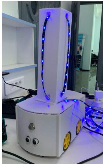
Figure III.22 Image of UV lamps installed in the prototype
