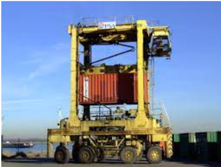
Figure I.19 Cavalier gerbeur (CG) [13] .
