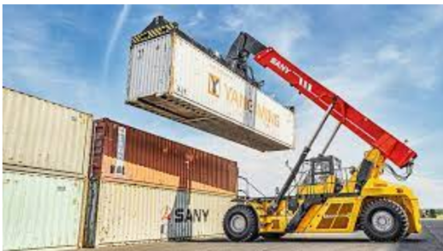
Figure I.17 Reach Stackers (RS) [11].
