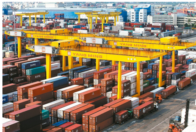
Figure I.15 Rail Mounted Gantry Crane (RMGC) [9].
