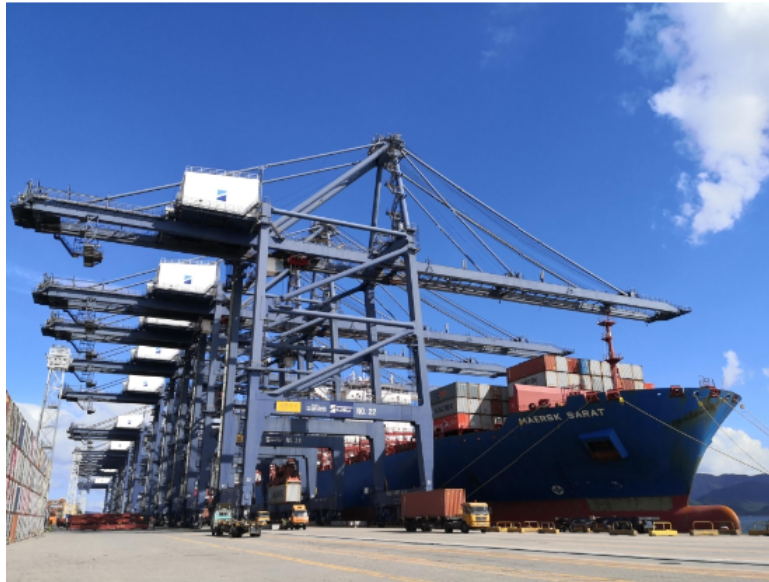
Figure I.14 Quay Crane (QC) [8].
