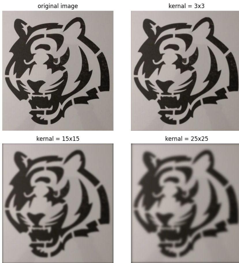
Figure 3.8 GaussianBlur with varying kernel values.
