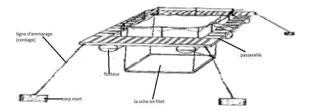
Figure II. 1: cage flottante
