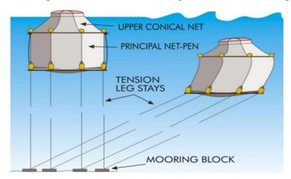
Figure II. 6: Démonstration d'une cage REFA tensions legs. (Refamed)
