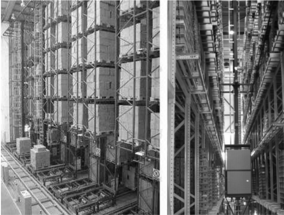
Figure 1.2: Automated Storage and Retrieval System (AS/RS)
