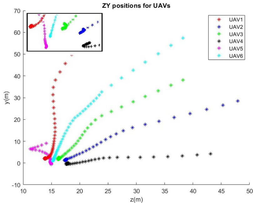
FIGURE 4.7: 2D targets and trajectory generated by PSO algorithm with collision avoidance
