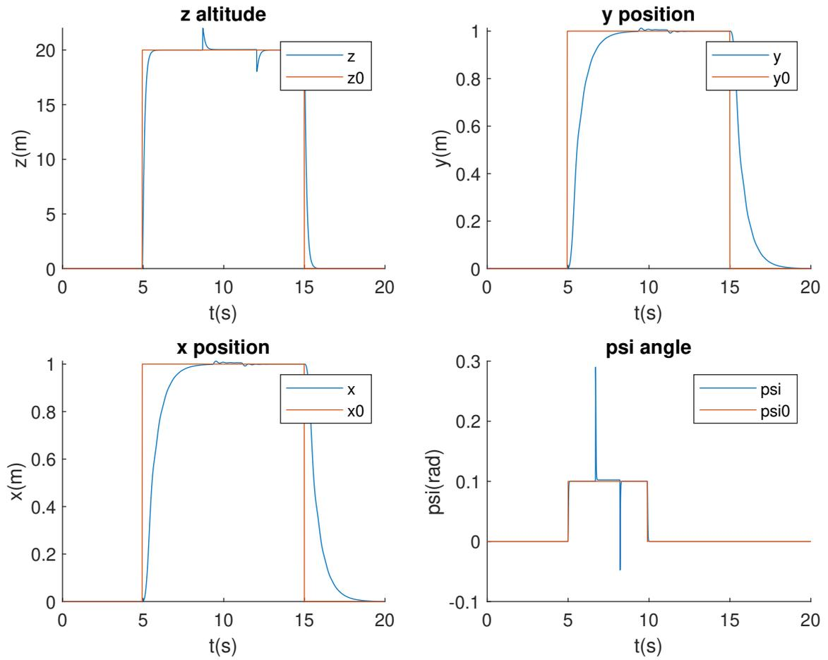
FIGURE 4.4: xyz positions and the yaw angle  $\psi$  with disturbances
