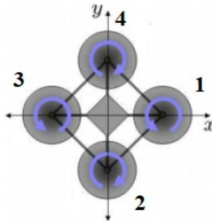
FIGURE 2.2: Direction of propeller's rotations
