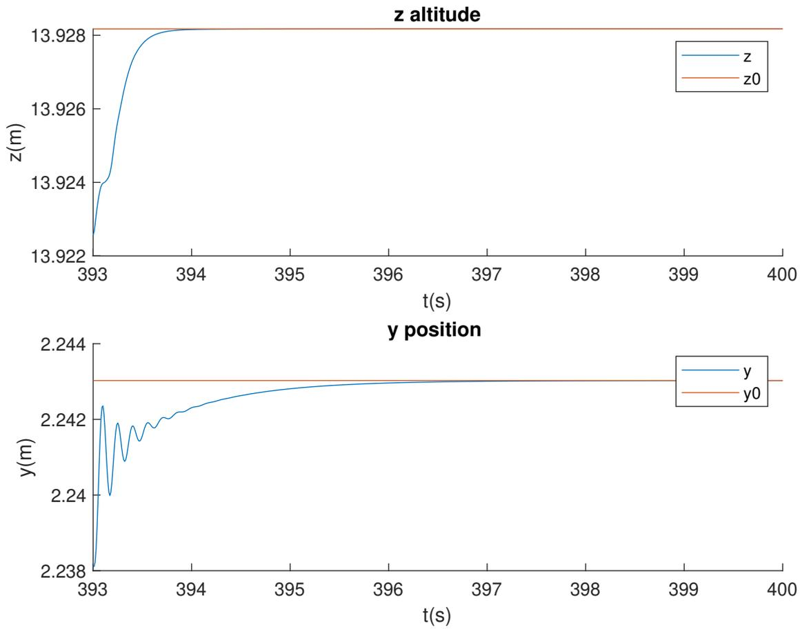
FIGURE 4.11: y and z positions for UAV1 between two time samples
