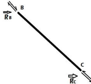
$$\vec{R}_B = -\vec{R}_C \quad \text{et} \quad R_B = R_C$$
