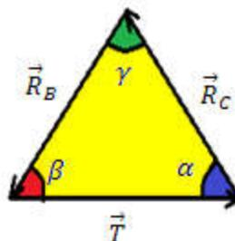
$$tg\alpha = \frac{130}{40} = 3,25 \Rightarrow \alpha = 72,89^\circ \quad \text{et} \quad tg\beta = \frac{130}{80} = 1,625 \Rightarrow \beta = 58,39^\circ$$
