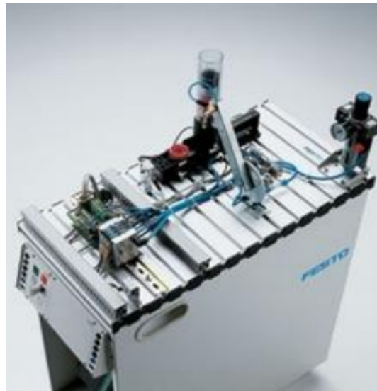
FIGURE 2.17 – Station de distribution[11]
