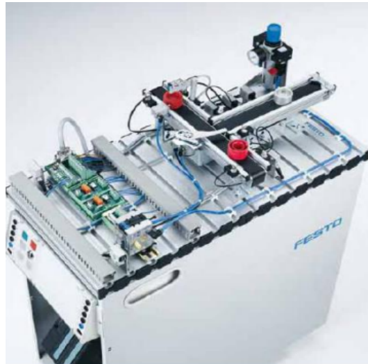
FIGURE 2.19 – Station de séparation[11]
