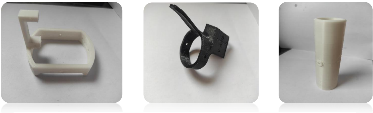
Figure 3. 9 printed parts of Outer gimbal, Inner gimbal and Motor tube
