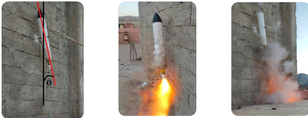
Figure 3.39 Second Static control test for pitch angle
