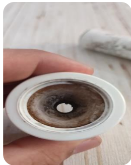
Figure 3. 13 Nozzle divergent section type 'd' made from cement formed with 3d printed mold
