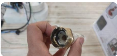
Figure 3. 4 Motor case contain propellants with circle grain form
