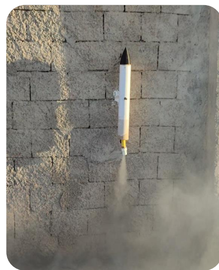
Figure 3. 38 First Static control test for pitch angle
