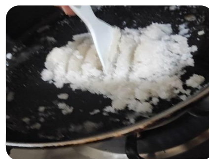
Figure 3. 25 Sugar Preparation and Mixing Motor Propellant
