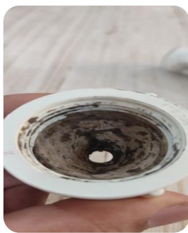
Figure 3. 14 nozzle convergent section type 'd' made from cement formed with 3d printed mold
