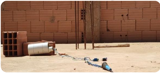
Figure 3. 37 Motor Static test with the nozzle
