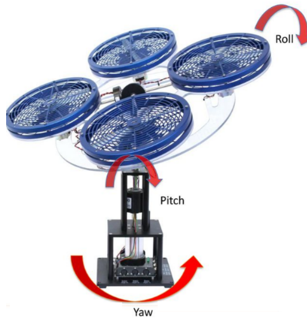
Figure 2.7. Structure de Quanser 3DDL
