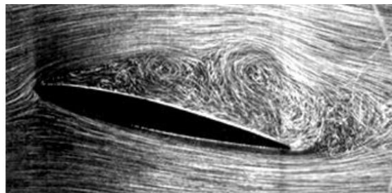
Figure III.26 Formation des tourbillons
