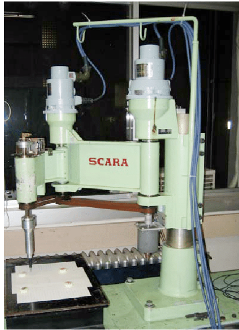
Figure 1.7: One of Hiroshi Makino's first prototypes of the SCARA structure
