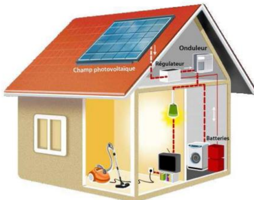
Figure II. 8: Système photovoltaïque autonome (Photovoltaïque –stockage).
