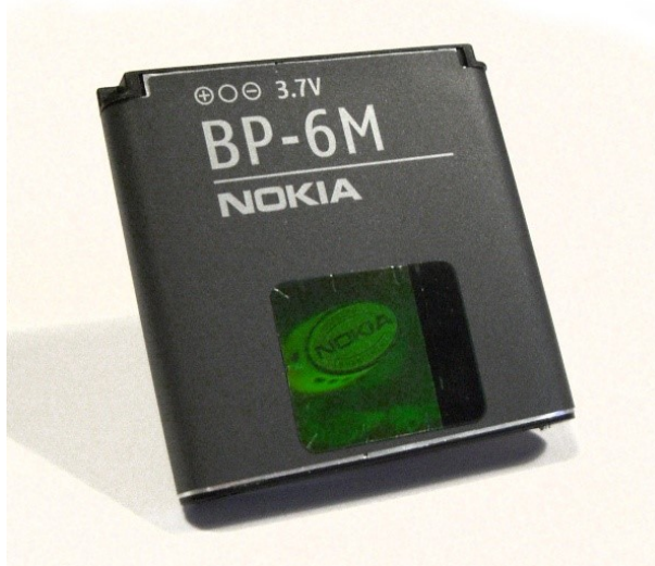
Figure 1.17: A rechargeable lithium polymer mobile battery
