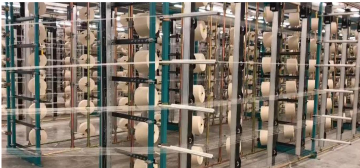
Figure 2. 17: BALL WARPING (Ourdissage). (1)
