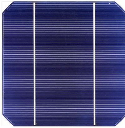
FIGURE I-7 CELLULE EN SILICIUM MONOCRISTALLIN.
