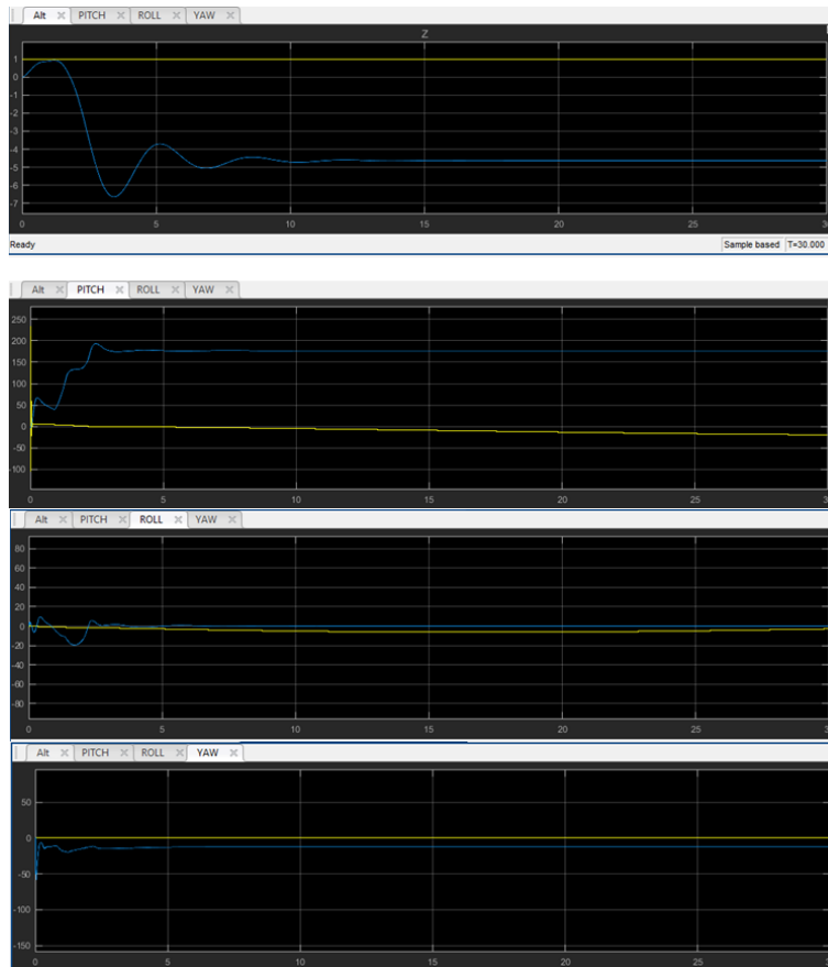
Figure 4.15: Outputs and inputs of the yaw,pitch, roll and altitude of the quadrotor on X configuration
