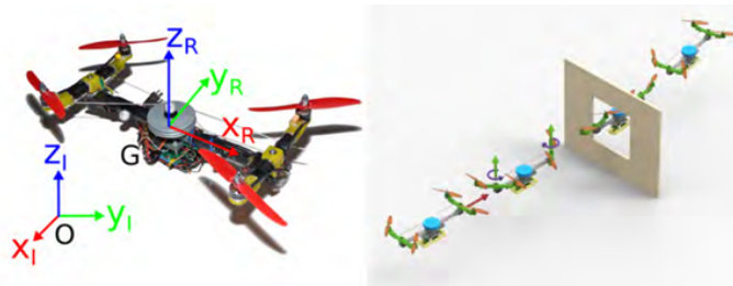
Figure 1.18: Horizontal pivoting arms drone [58]
