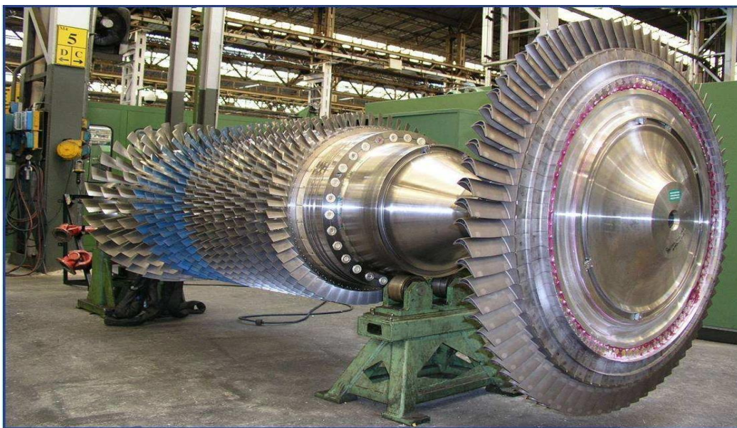
Fig 2.9: HP rotor of the MS5002C gas turbine
