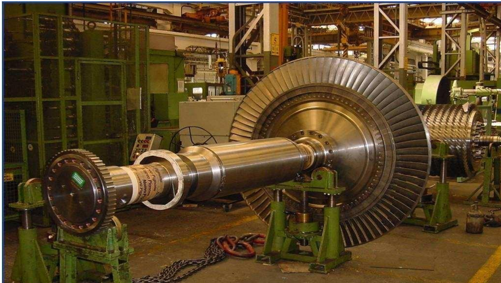
Fig 2.10: LP rotor of the MS5002C gas turbine [2]
