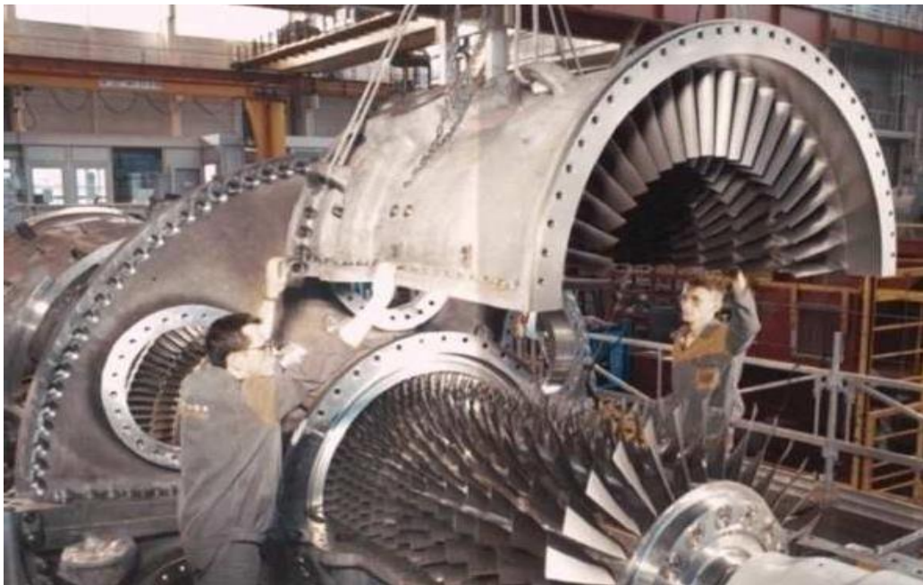
Fig 2.3: Stator of the axial compressor
