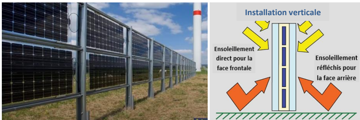
Figure 2.8 : Panneau bifacial vertical [38].
