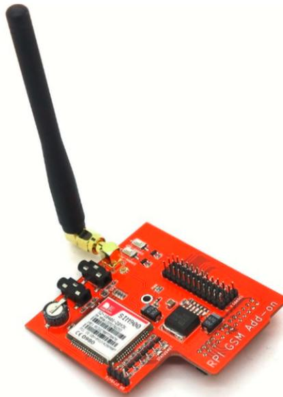
FIGURE 3.3 – Raspberry Pi SIM900 GSM/GPRS ADD-ON
