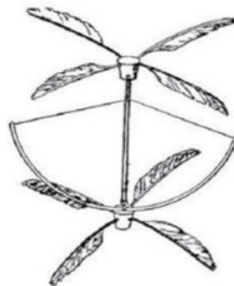
(b) Contra-rotating propeller, Launoy and Bienvenue
