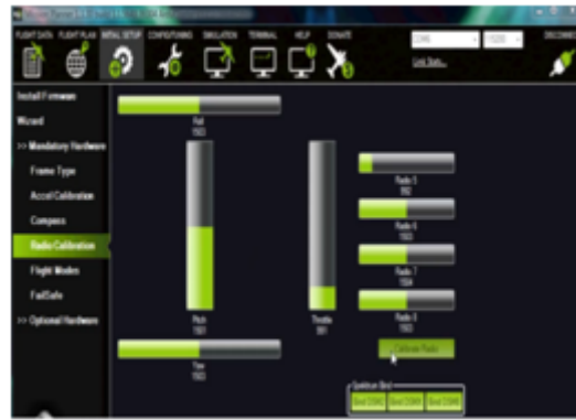
FIGURE 4.14: Calibration de la radio-commande
