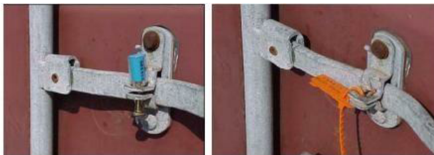
Figure 9: conteneur PLEIN et conteneur VIDE.
